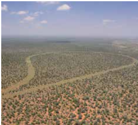
Bush cleared for the rapid loading rail loop at the mine.
